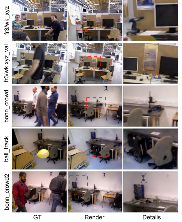
Fig. 3. Qualitative mapping results in dynamic environments. The third column presents magnified details of the regions highlighted by red dashed boxes in the rendered images, demonstrating the high-fidelity reconstruction of the static background after dynamic object removal.
